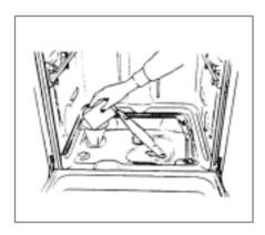
The salt container should be filled after about every 30 wash cycles.
